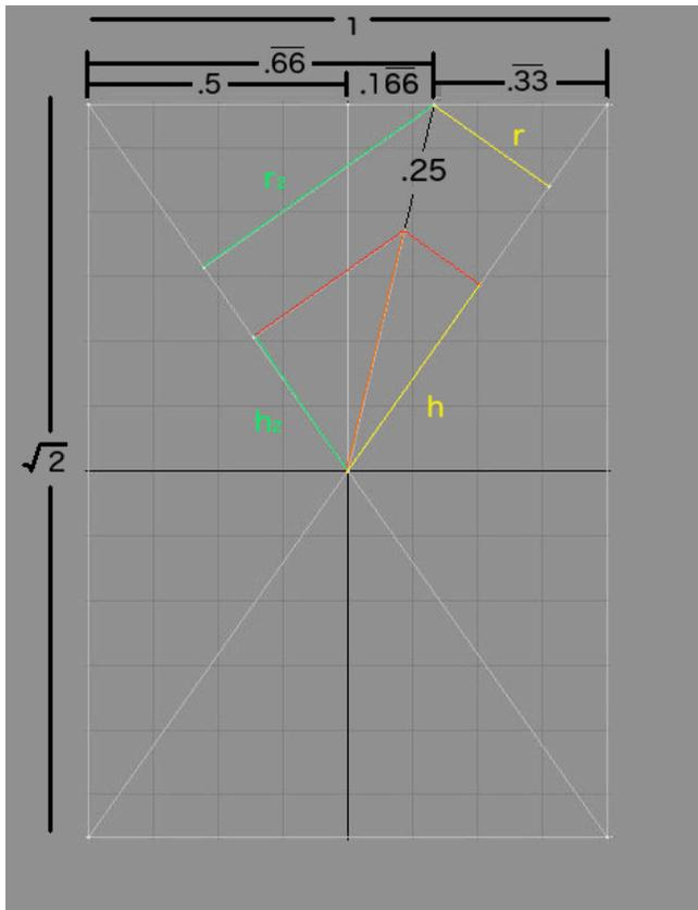
We have reduced the height of our original orange line by .25 units. And from this reduced height, we have drawn lines parallel to  $r$  and  $r_2$ . Subtracting .25 from the original OrangeLine, we get ShortOrangeLine = 0.47648 units. And since the angles have remained unchanged, we can calculate  $h$  and  $h_2$ .
