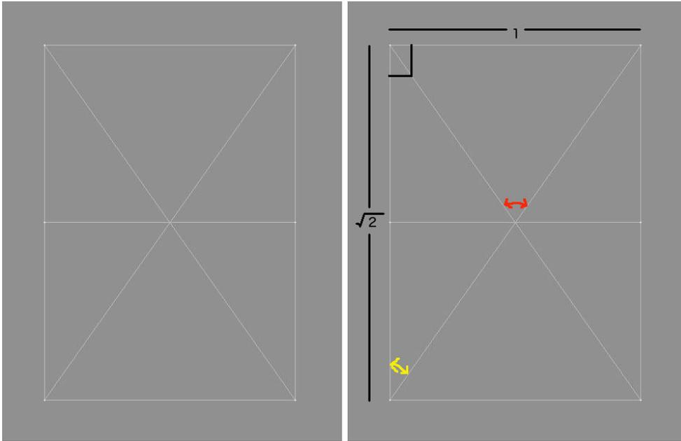
From the view above, it starts to become apparent that the angle of intersection (shown in red) between the axes of rotation is not perpendicular. So, how do we calculate the angle of intersection? First, we need to ascribe units to our cube. If we agree that our cube is one unit long by one unit wide by one unit tall, then we can begin to figure out the angle of intersection.
