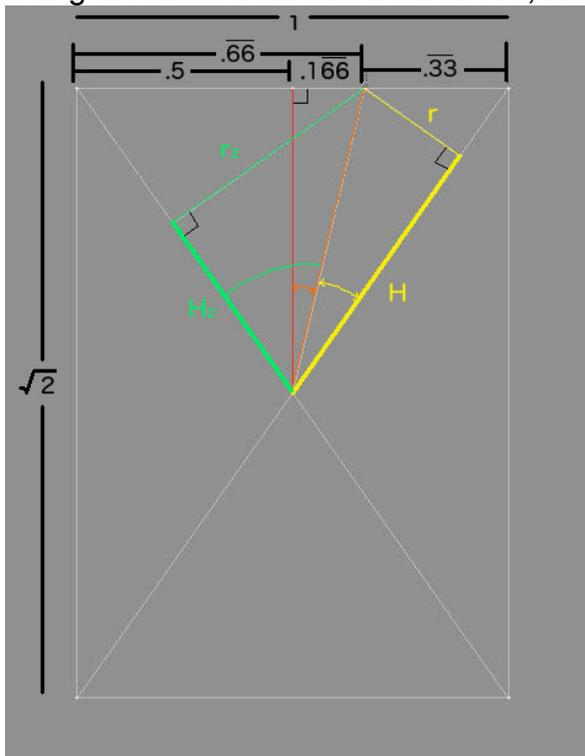
In the drawing above, the orange line segment represents the angle where the two gears are going to meet at their pitch circles. The yellow line (r) represents the radius of the pitch circle of the smaller gear. The green line (r2) represents the radius of the pitch circle of the larger gear. We want to solve for r and r2.
