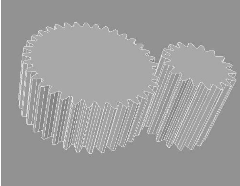
So, how do we turn these two gears into beveled gears? One easy way is to select all the points on the bottom of each gear and set them all to 0,0,0 which results in gears like in the photo below:
