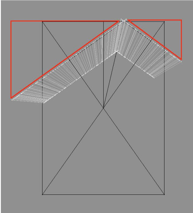
With the gears cut off and rotated in position, they will properly rotate around their axis of rotation and mesh with each other. Great! But, we still need more material out to where the red example lines are and beyond. Now, one cool thing about triangles and conical sections, is that when scaled up, a slice at a given elevation will retain the same scale. What? No matter how much scale up our gears, the slices that we need will keep their same geometry. Look at the picture below:
