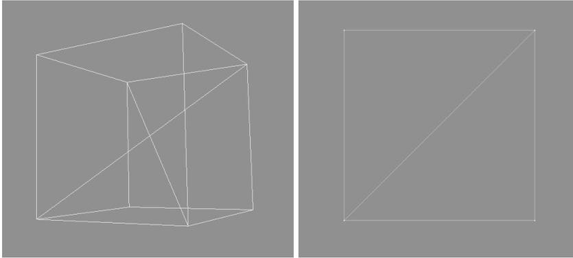
From the side view, it becomes clear that the plane, upon which the axes of rotation reside, is at a 45 degree angle and it runs from the bottom front of the cube to the top back of the cube. To get a better view of the axes of rotation, let's rotate our cube 45 degrees so that the plane on which the axes of rotation resides is now vertical. Below on the left shows the rotated cube from perspective and on the right shows the rotated cube from the right:
